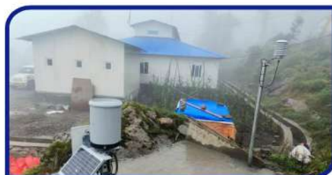
AUTOMATIC WEATHER STATION AT PROJECT SITE
